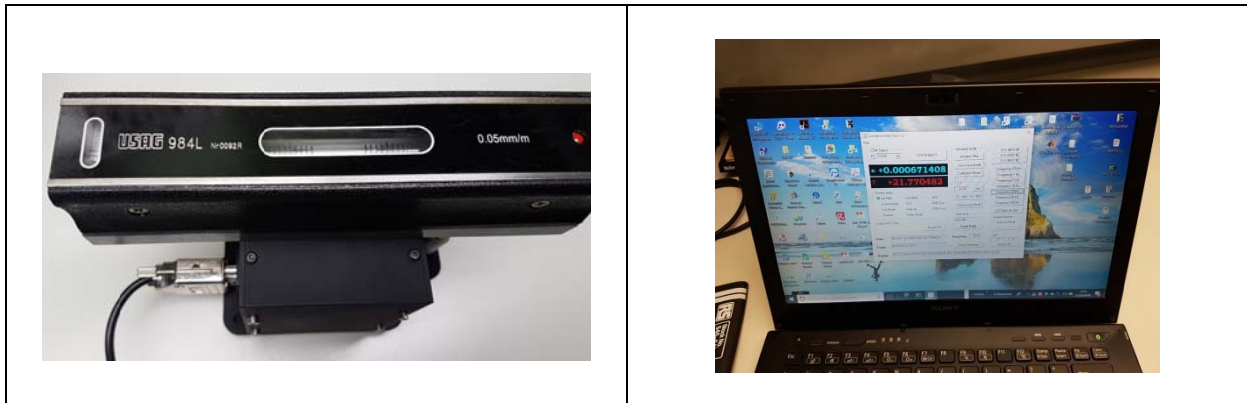
Figure_9 In the figures are shown the pictures of the calibration facility with a precise level and the display of the accelerometer exit, so to verifying the correctness of the close to zero exit when it's axis is in an horizontal pane.
