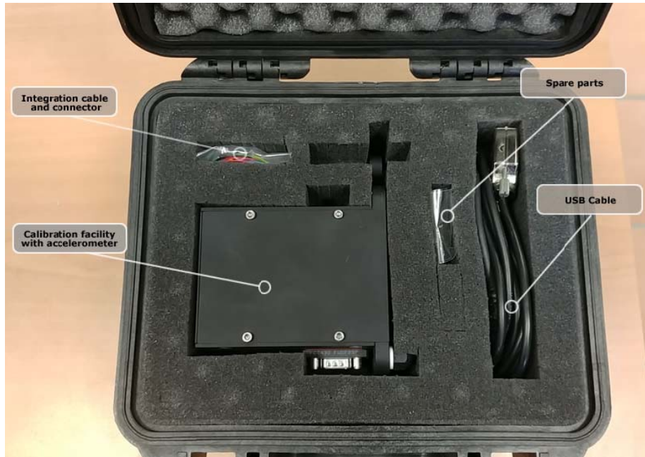
Figure_2 In the following figure is shown the hardware parts placed inside of the transport case.
